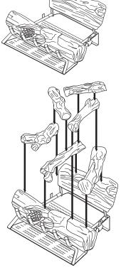
Figure 8 - Installing Logs
